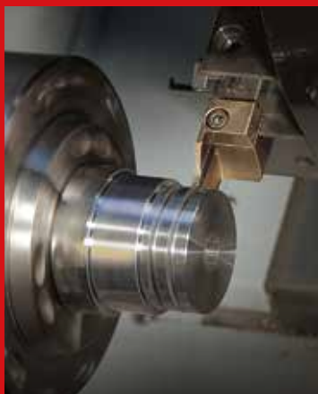
Tools and inserts for parting and grooving
