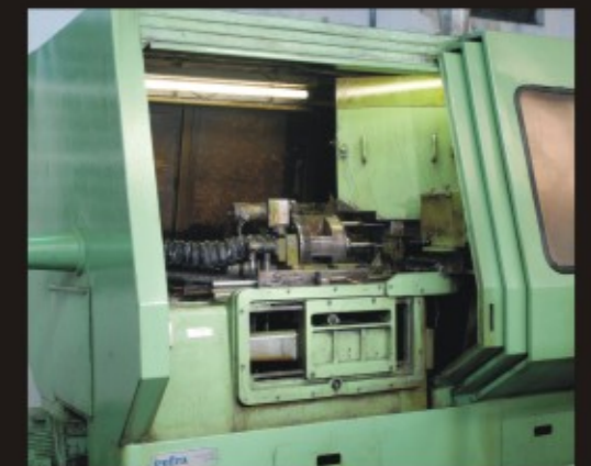
HIGH PRODUCTIVITY AUTOMATIC FLUTE GRINDING MACHINE
